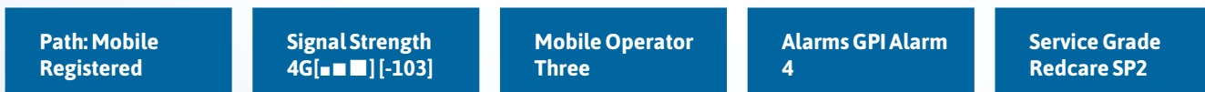
Figure 6 – Typical display cycling on a fully commissioned unit with a good signal strength and Pin 4 in the alarm or open state.
