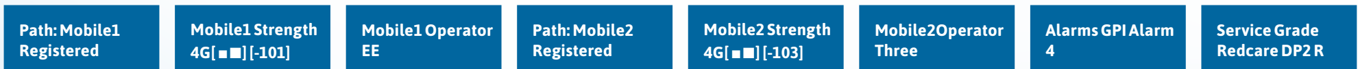
Figure 6 – typical display cycling on a fully commissioned unit with a good signal strength and Pin 4 in the alarm or open state.
