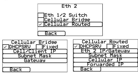
By default the Cellular Routed mode is selected, with Forwarded IP (i.e. the address of the attached device) set to 192.168.1.1 and the Gateway IP (i.e. the address of the Eth2 connection on the terminal) set to 192.168.1.254. The DHCP server is on by default.
